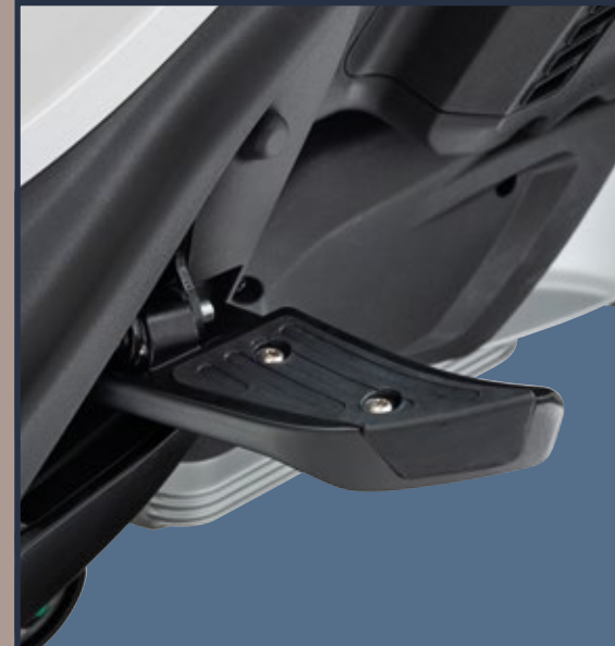
RETRACTABLE PASSENGER FOOTPEGS
