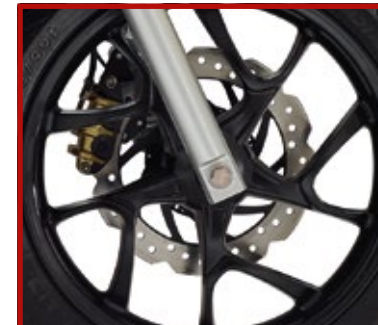
BRAKE DISCS WITH WAVY PROFILE
